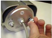
Do NOT lose the cap, you will need to replace the weather-proof cap after adjustment
